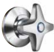
CM 101E Exposed part for flush cock half turn cross handle 25 mm (1") consisting of operating lever, cartridge sleeve and wall flange (suitable for CFC 102)
