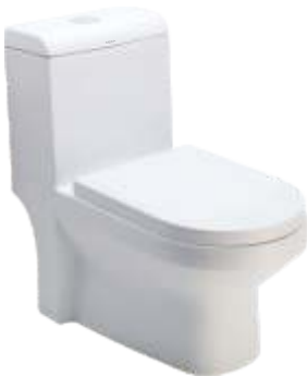
CAPSTAN 2068 One Piece EWC S Concealed P trap: 715 x 380 x 810 mm S trap: 715 x 375 x 795 mm 2368 Soft Close Seat Cover 2268 Twin Flush Fittings Available in • Wall distance 255 +10 mm • P trap
