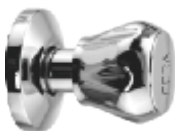
CQ 651E Quarter Turn CC 151E Half Turn Exposed part for flush cock 25 mm (1") consisting of operating lever, cartridge sleeve and wall flange (suitable for CFC 102)
